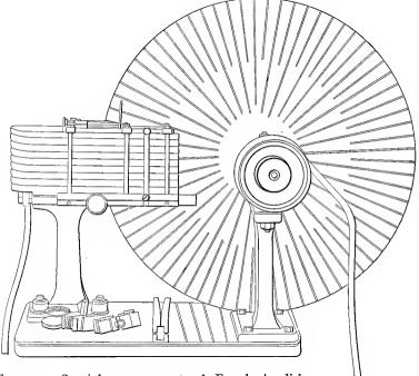
FIG. 20. Special arrangement of Faraday's disk or Barlow's wheel for demonstration and experiment.
